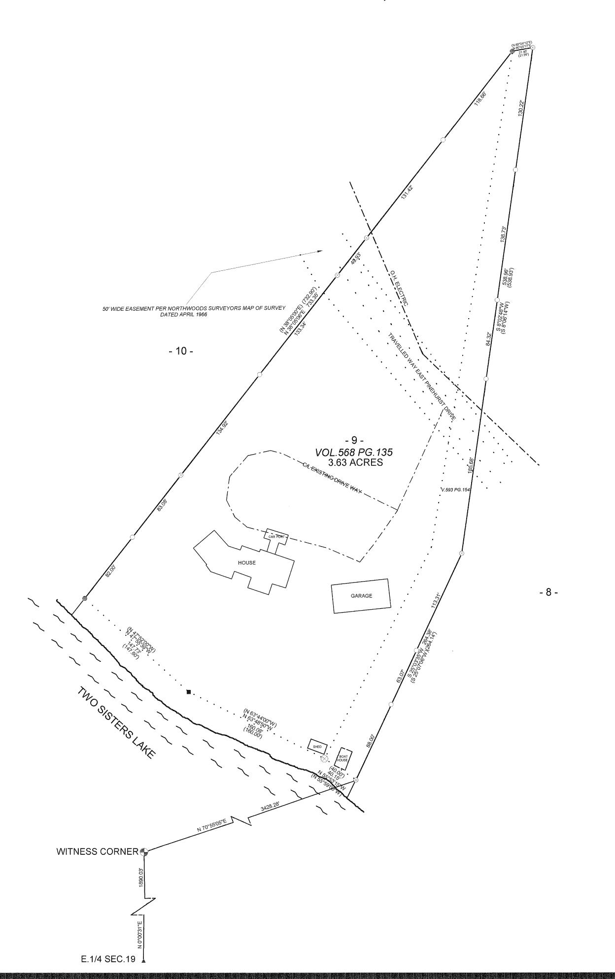
NOTE: THE AREA SHOWN REPRESENTS THE COMBINED PARCELS DESCRIBED IN VOL.568 PG. 135 AND VOL. 593 PG.154 AS RECORDED IN THE ONEIDA COUNTY REGISTER OF DEEDS. THE PURPOSE OF THIS SURVEY IS TO COMBINE PARCELS DESCRIBED IN VOLUME 568 PG. 135 AND VOLUME 593 PG. 154 INTO ONE DESCRIPTION AREA SHOWN DOES NOT INCLUDE LANDS BETWEEN THE MEANDER LINE AND THE ORDINARY HIGH WATER MARK OF TWO SISTERS LAKE.
