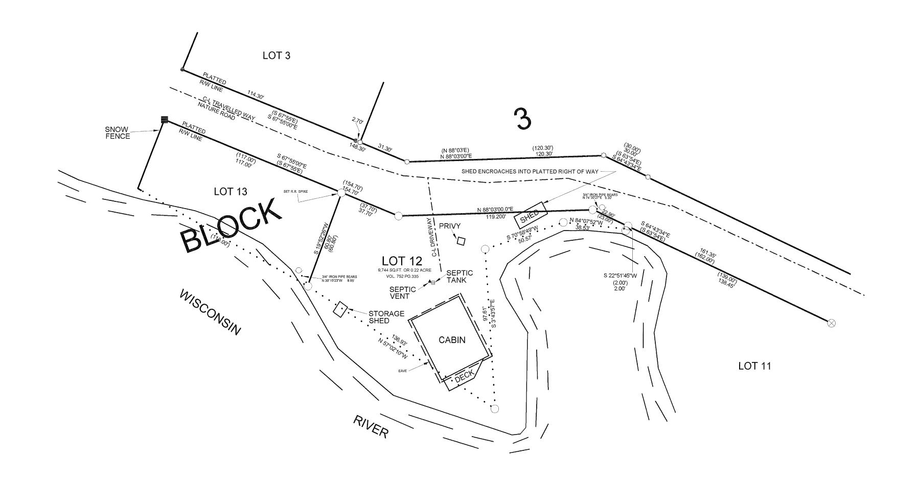
Area does not include the lands between the meander line and the bank of the Wisconsin River. Set railroad spike for NW corner of lot 12. Platted road right of way width appears to be +-33' based on monumentation found in the field.
