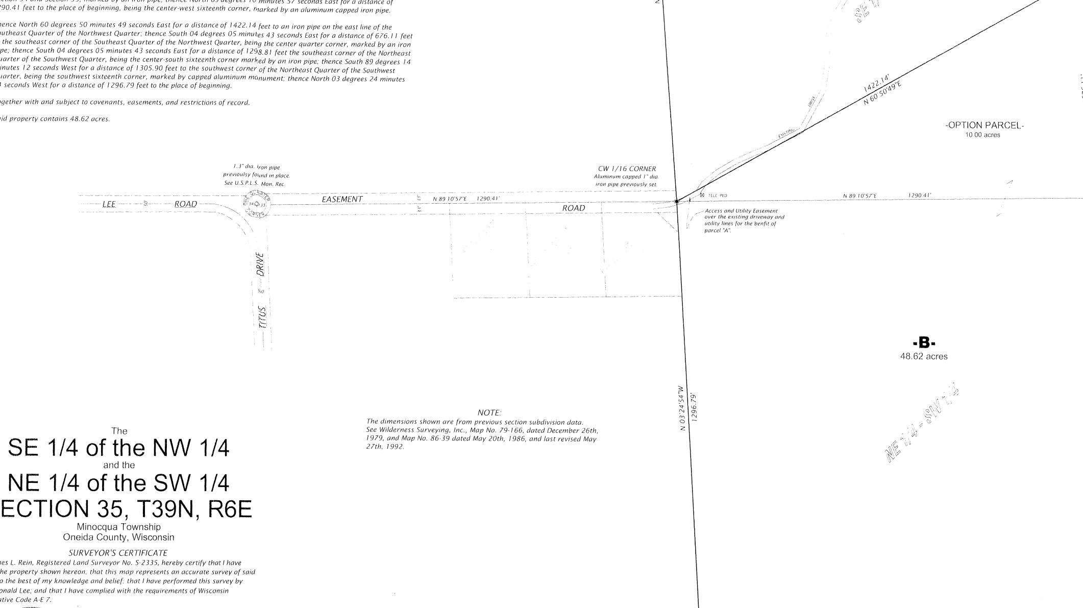
Bearing base assumed, referenced to the north line of the SE 1/4 of the NW 1/4 bearing, N88'24'24"E LEGEND  $\bigcirc$  = Iron pipe set, 1" dia. x 24" long.
