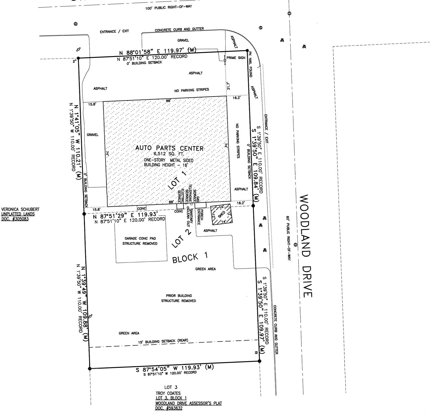
BEARINGS ARE BASED ON THE WEST RIGHT OF WAY
