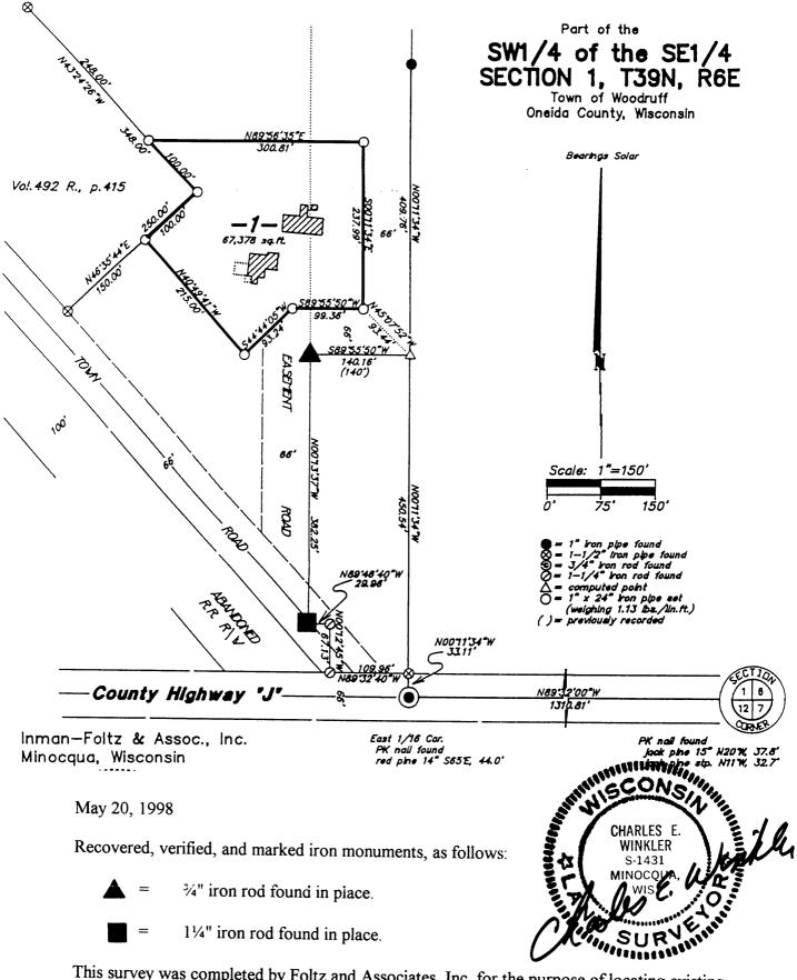
This survey was completed by Foltz and Associates, Inc. for the purpose of locating existing corners by the order of Bill McCutchin, who has executed a written waiver for all other requirements of Wis. Adm. Code Chap. A-E 7. A closed traverse was not made and the minimum accuracy is 1 part in 100 and plus or minus 2°.
