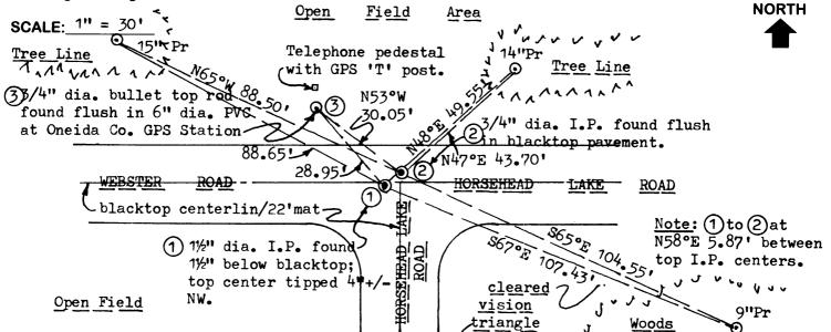
Unless otherwise indicated, all bearing tree ties are to a .25" dia. by 2.5" long PK nail with a 1.25" dia. steel washer driven into unblazed right face and a .25" dia. by 2.5" long PK nail with a 2" dia. steel washer stamped 'BT' is also driven into unblazed face of bearing tree at DBH; the basis for measured bearings is magnetic to nearest degree and all tie distances are horizontal measure to nearest 1/100th feet.
