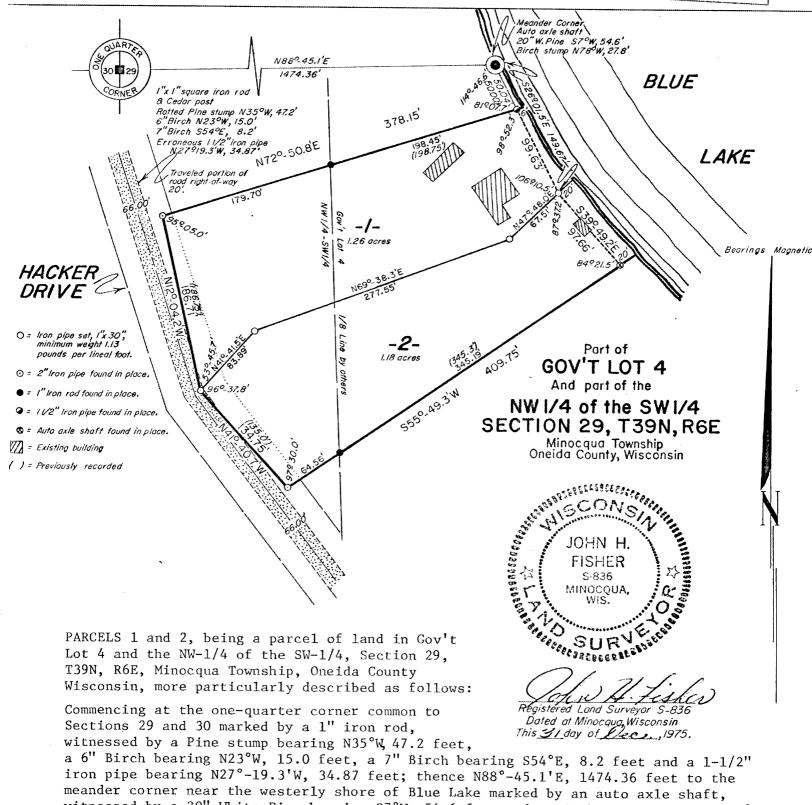
27.8 feet; thence S26°-01.5'E, 50.04 feet along the lake to the place of beginning, marked by a 1-1/2" iron pipe.
