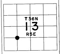
Plan view map of survey landmark location with bearing and distance ties to a minimum of four(4) described witness or reference monuments of concrete, natural stone, metal, live bearing trees or equivalent material and/or by described GPS method and precision.
