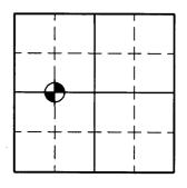
Plan view map of survey landmark location with bearing and distance ties to a minimum of four(4) described witness or reference monuments of concrete, natural stone, metal, live bearing trees or equivalent material and/or described GPS method and precision.
