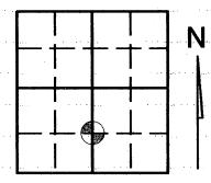
Plan view map of survey landmark location with bearing and distance ties to a minimum of four (4) described witness or reference monuments of concrete, natural stone, metal, live bearing trees or equivalent material and/or by described GPS method and precision.
