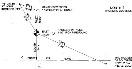
MAG NAIL SET IN TOP OF SOUTH END OF NEW 12" DIA H.D.P.E. CULVERT PIPE
