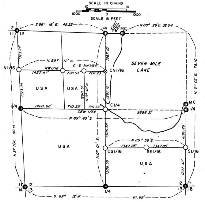
Bearings and distances on outside perimeter of section are from 1941 dependent resurvey. Note:
