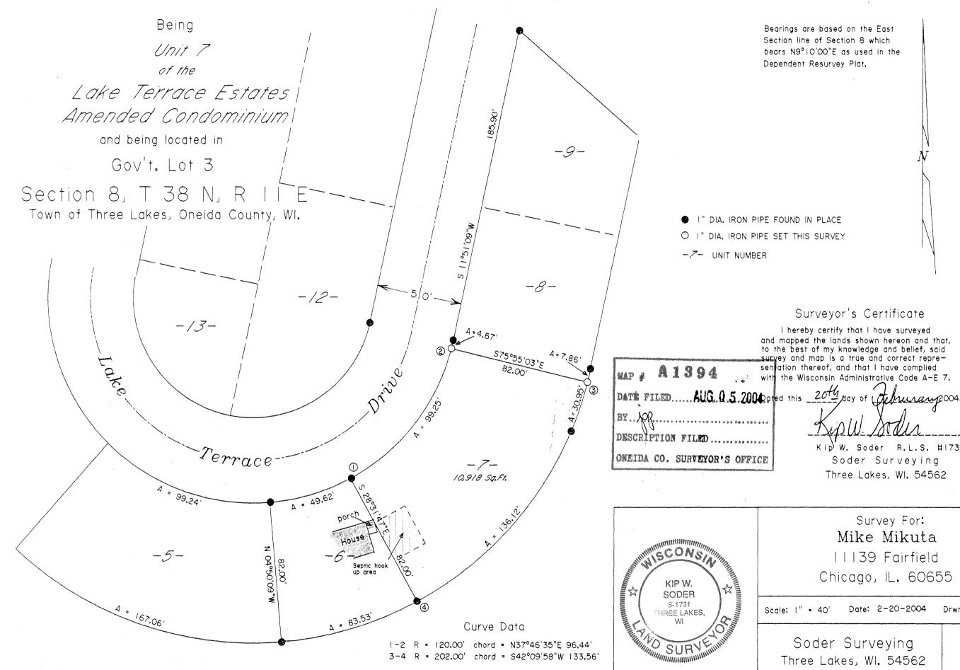
Bearings are based on the East Section line of Section 8 which bears N9°10'00"E as used in the Dependent Resurvey Plat.
