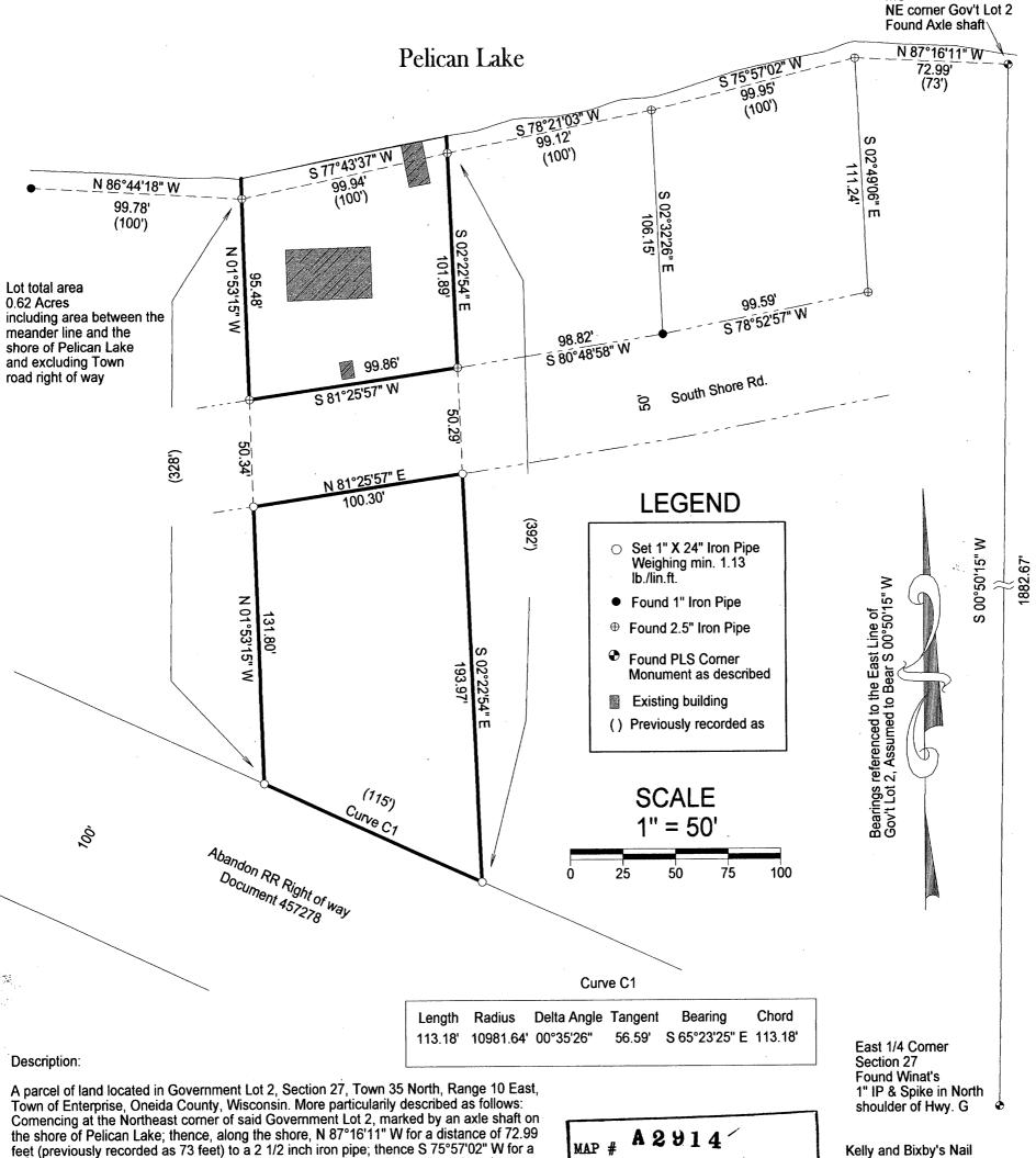
Comencing at the Northeast corner of said Government Lot 2, marked by an axle shaft on the shore of Pelican Lake; thence, along the shore, N 87°16'11" W for a distance of 72.99 feet (previously recorded as 73 feet) to a 2 1/2 inch iron pipe; thence S 75°57'02" W for a distance of 99.95 feet (previously recorded as 100 feet) to a 2 1/2 inch iron pipe; thence S 78°21'03" W for a distance of 99.12 feet (previously recorded
