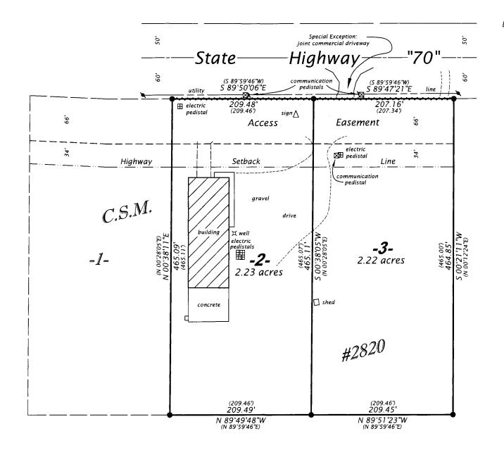
Bearings Oneida County Grid, based on GPS survey data, referenced to the east line of Lot 3, C.S.M. #2820 bearing \$ 00°21'11"W.
