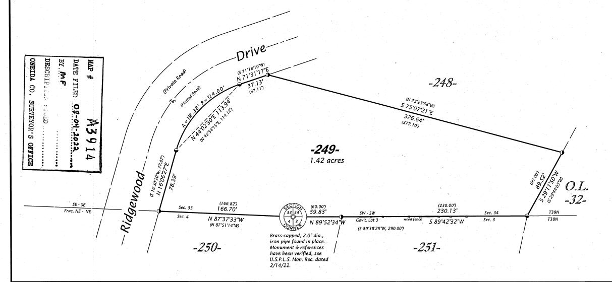
Bearing base is assumed, referenced to the northerly line of Lot 249, Timber Ridge II, bearing S 75'07'21"E.
