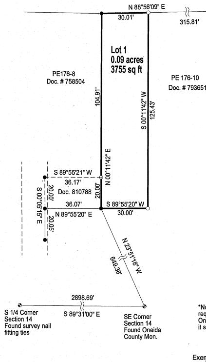
Bearings referenced to the South line of Section 14, Assumed to bear S 89°31'00" **SCALE**
