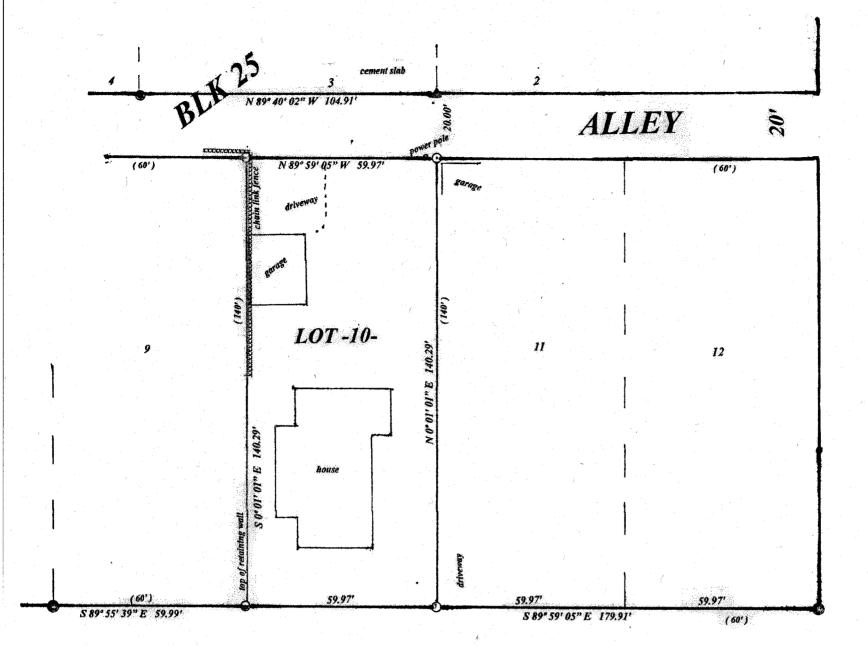
North is referenced to the West line Lot I CSM. v. 20, p. 4336 being a platted bearing of N 0° 06' 52" W.
