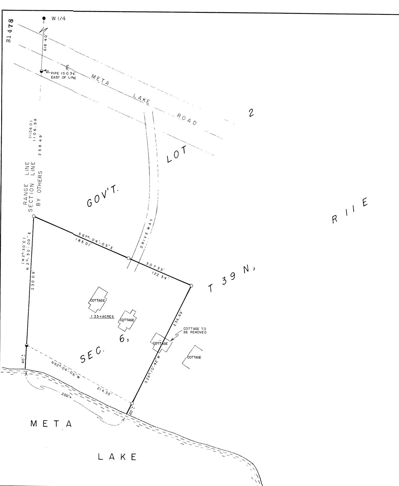
BEARINGS ARE BASED ON THE WEST SECTION LINE BEARING
