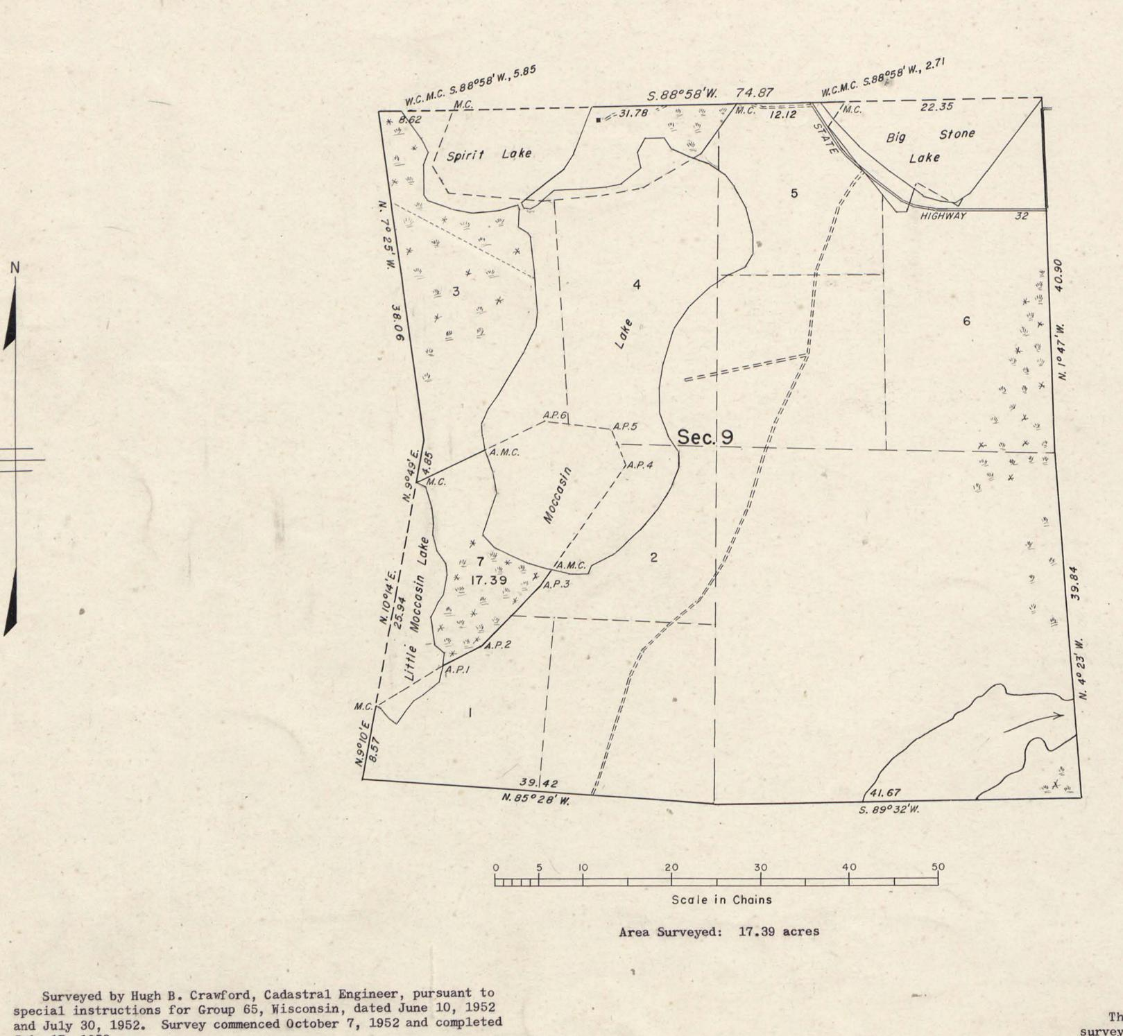
This plat represents a retracement and reestablishment of portions of the original subdivisional lines designed to restore all corners on the boundaries of Sec. 9 in their original locations according to the best available evidence, and the survey of omitted lands which were erroneously omitted from the original survey and not shown upon the plat approved December 20, 1859.
