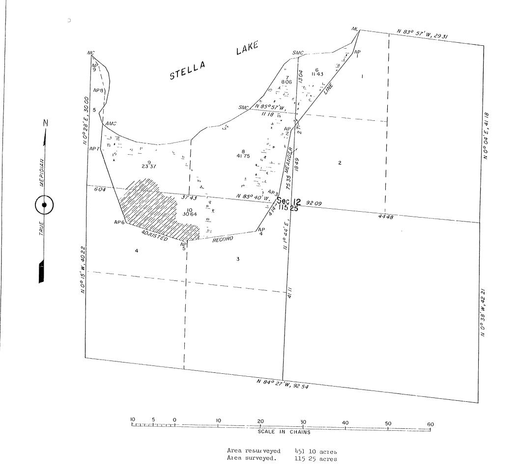
This plat represents a retracement and reestablishment of the original surveys designed to restore all corners on the boundaries of sec 12 in their original locations according to the best available evidence, and an extension survey to include lands .ich were erroneously omitted from the original survey and not shown upon the plat approved March 18,
