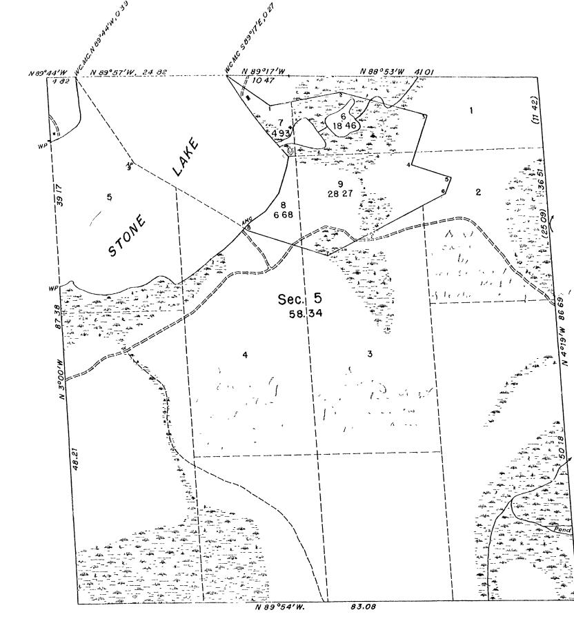
This plat represents the retracement and reestablishment of a portion of the township boundary and subdivisional lines, designed to restore all corners on the boundaries of sec. 5 in the true original locations according to the best available evidence of the position of the original corners, and an extension survey to include lands erroneously omitted from the original survey and not shown upon the plat approved June 9, 1864.
