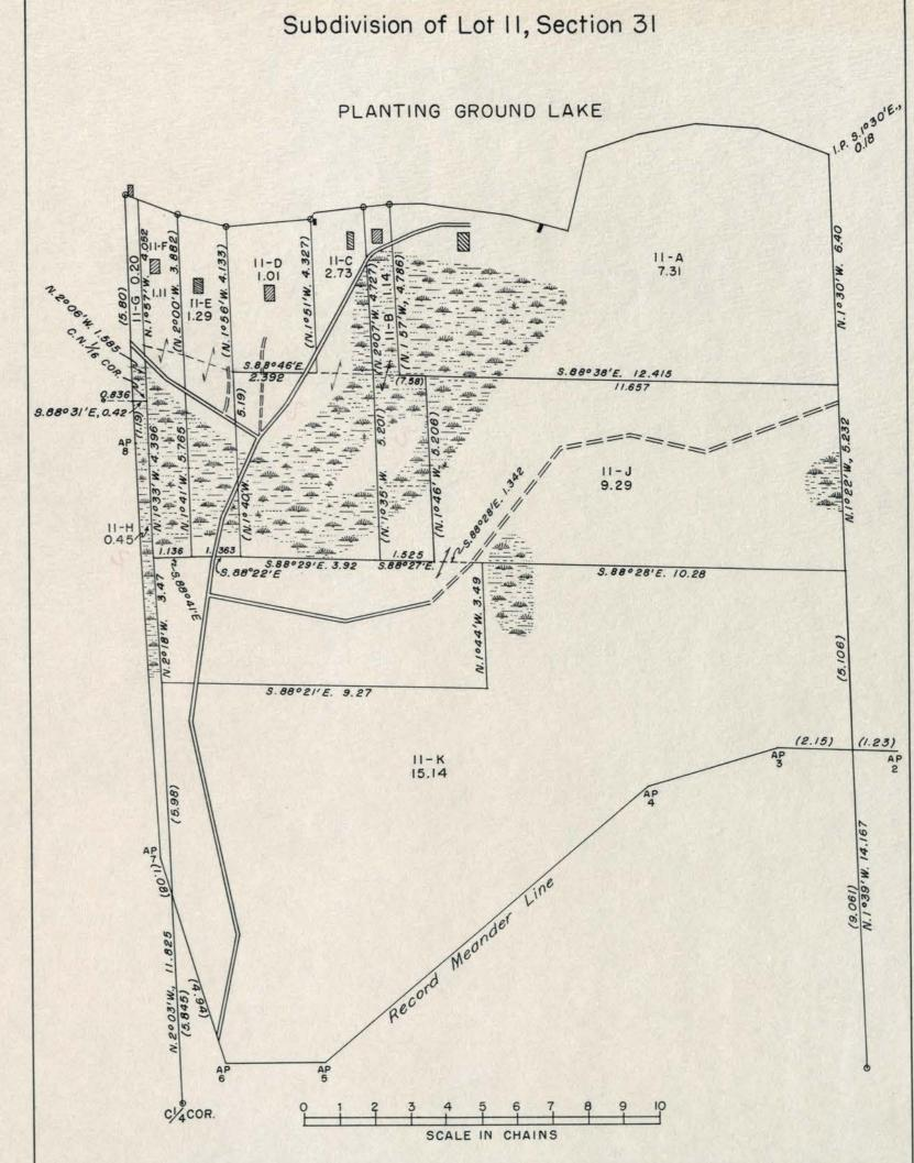
This plat represents a retracement and reestablishment of the boundaries of sec. 31, designed to restore the corners in their original locations according to the best available evidence, and the survey of public lands which were erroneously omitted from the original survey and not shown upon the plat approved February 4, 1860.
