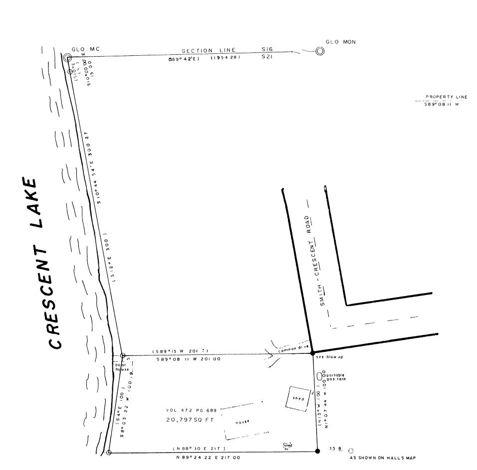
North is referenced to the North line of section 21 being a recorded bearing of S 89042' L.
