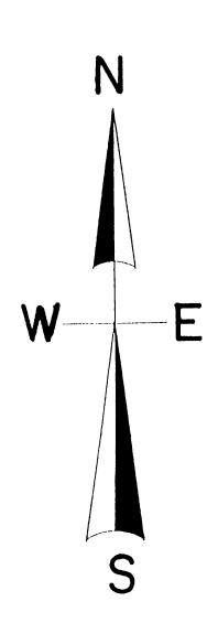
North is referenced to the North line of the NW.1, Sec. 28, being an assumed bearing of N 89° 25' 00" W.
