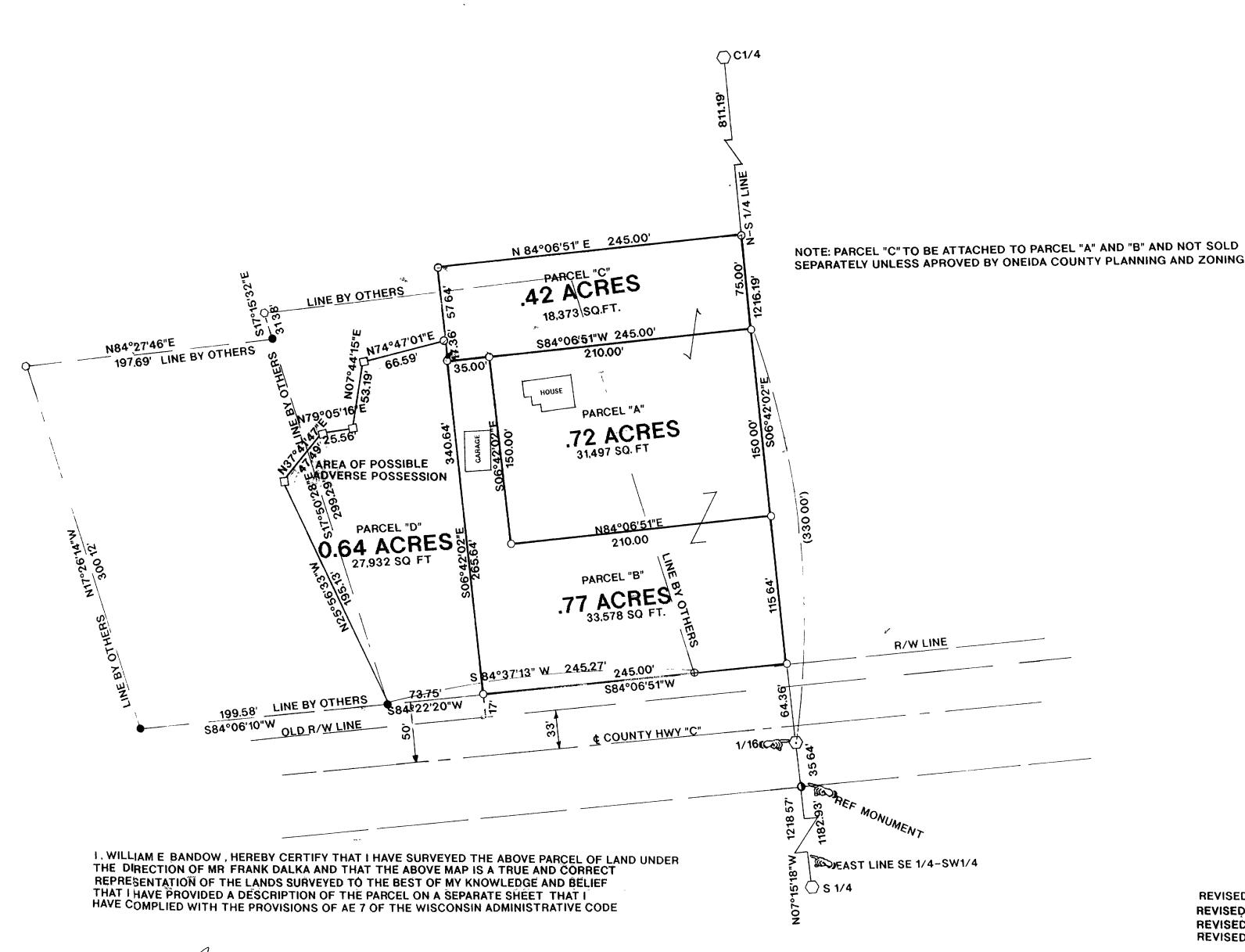
BEARINGS REFERENCED TO THE EAST LINE OF THE SE 1/4-SW 1/4, T37N, R9E ASSUMED TO BEAR NO7°15'18"W.
