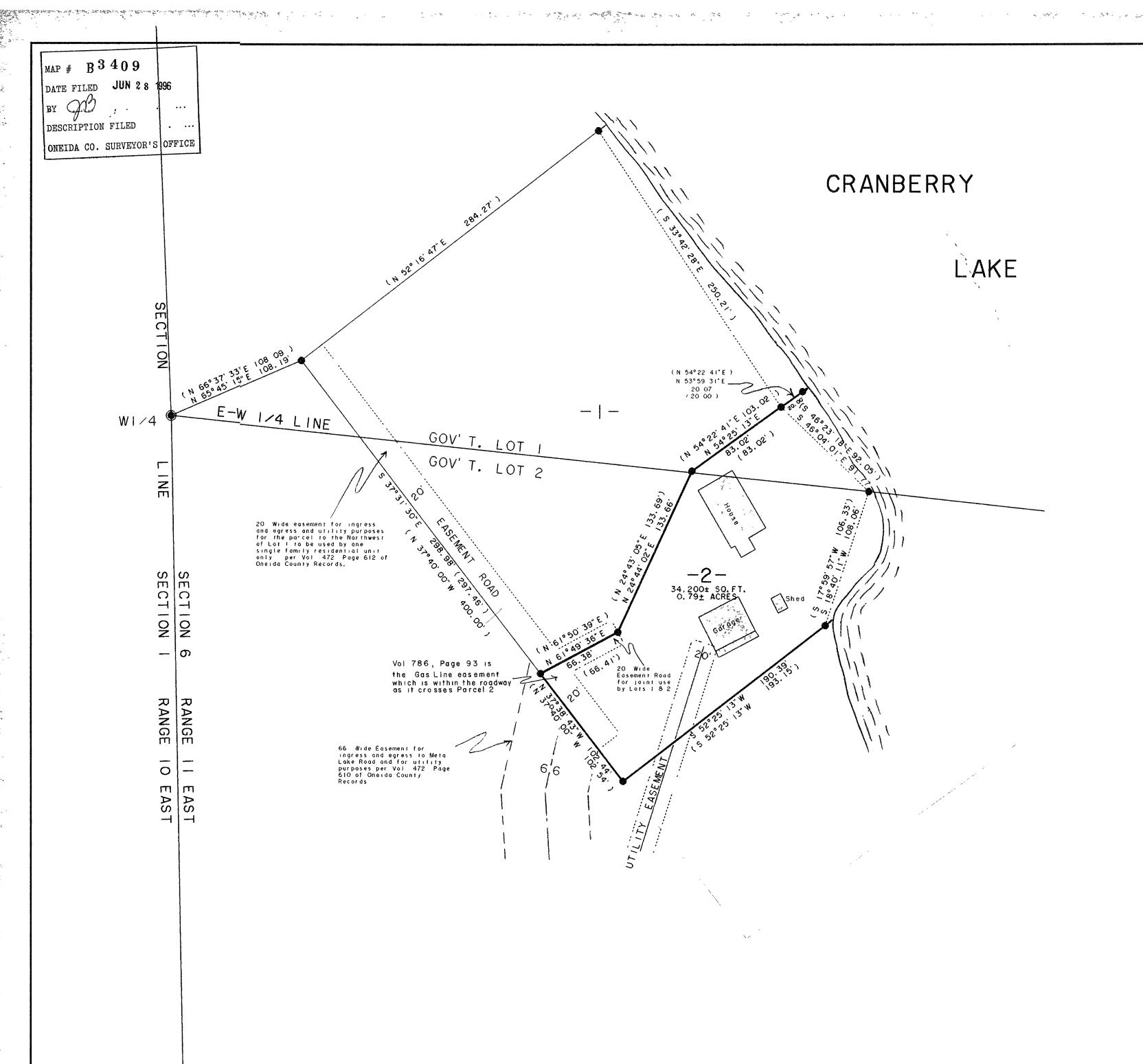
NOTE: Bearings are based on the South Line of Lot 2 of Certified Survey record in Vol. 3CSM, Page 892 of Oneida County Records with a bearing of S 52925'-13" W.
