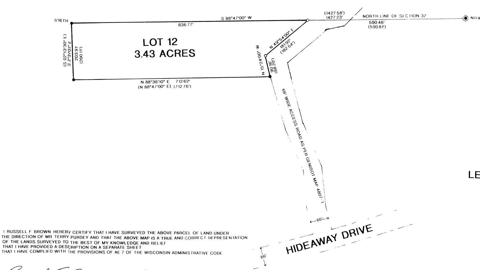
BEARINGS REFERENCED TO THE NORTH LINE SECTION T39 R9E ASSUMED TO BEAR S 88°47OO W
