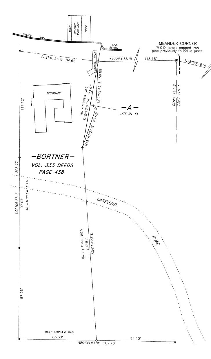
Bearings true based on a solar observation by Borthwoods Survveyors, Inc. referenced to the west line of the W 1/2 of the NE 1/4 Section 10, bearing S00°08'00"E
