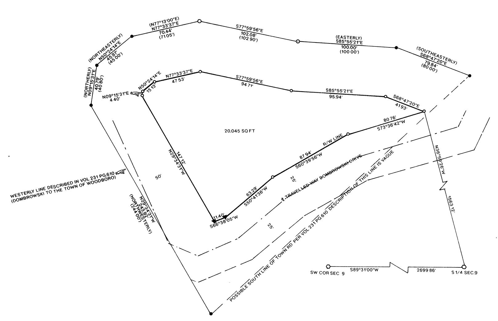
BEARINGS REFERENCED TO THE SOUTH LINE OF SECTION 9 T36N . R7E . ASSUMED TO BEAR S89°31'00"W
