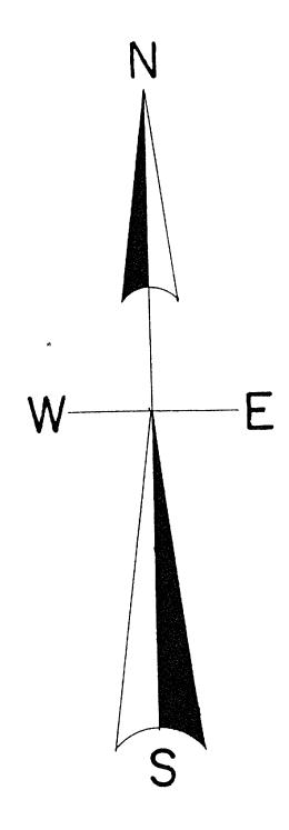
North is referenced to the West line CSM. V. 6, P. 1699, being a bearing Of N 1° 25' 20" W.
