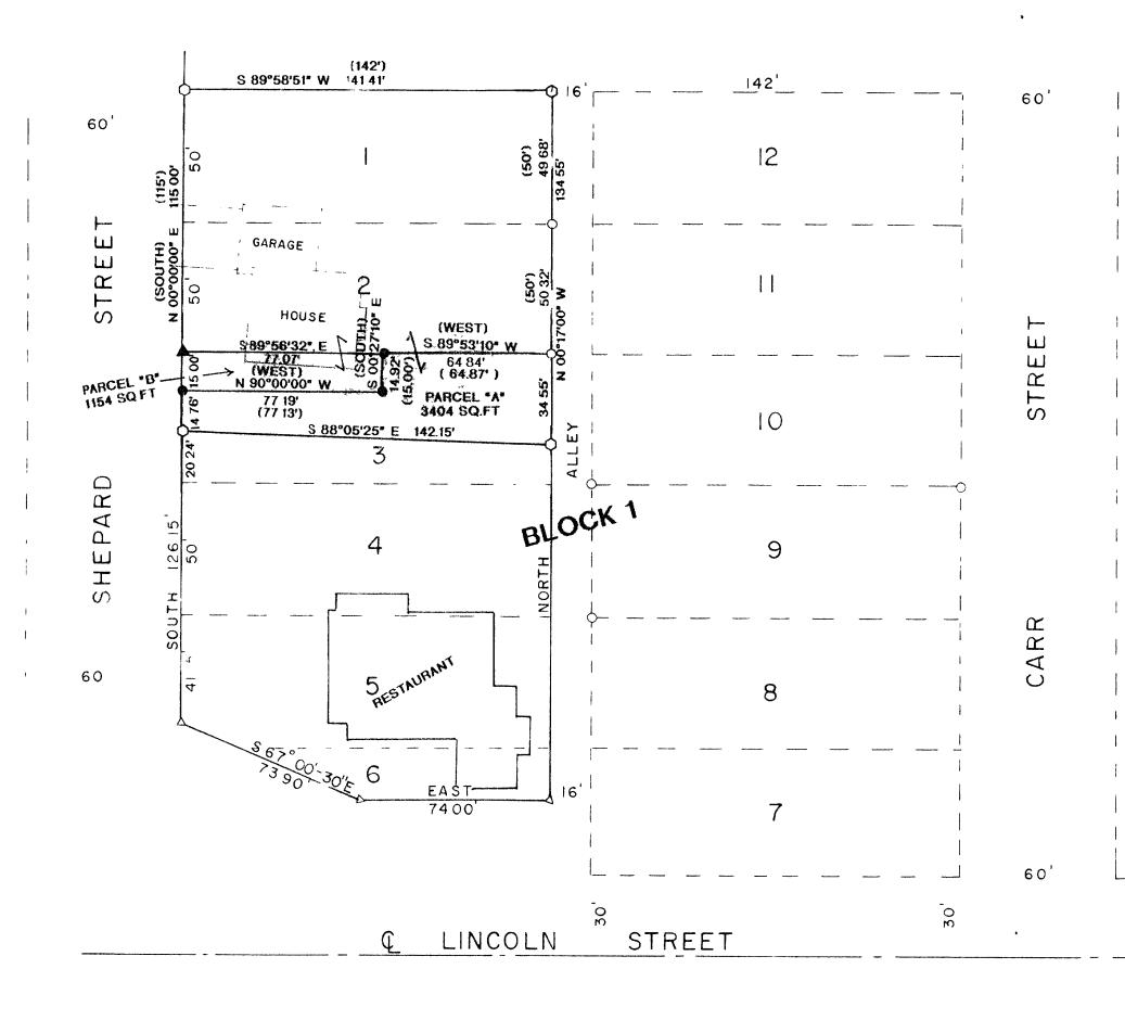
BEARINGS REFERENCED TO THE WEST LINE OF BLOCK 1, COHN, BING & SLIMMERS SECOND ADDITION TO THE CITY OF RHINELANDER ASSUMED TO BEAR S 00°00'00" E
