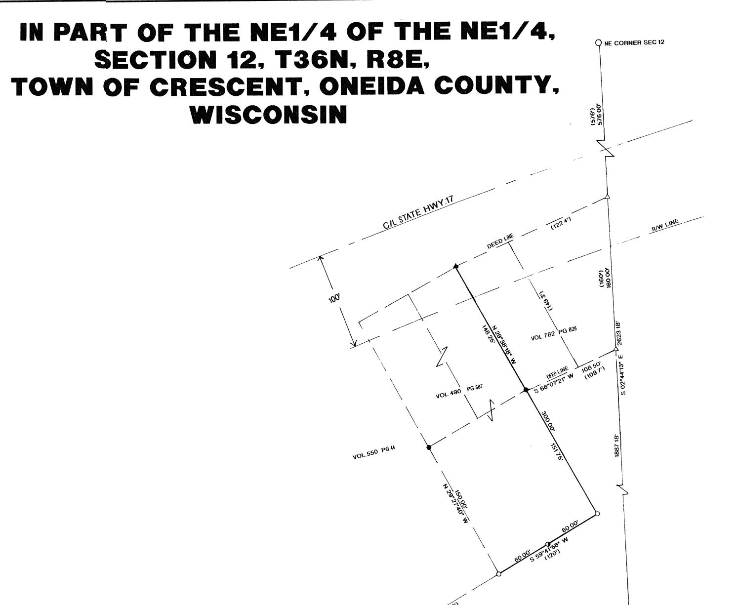
BEARINGS REFERENCED TO THE EAST LINE OF SECTION 12 T36N, R8E ASSUMED TO BEARS 02º4413º E
