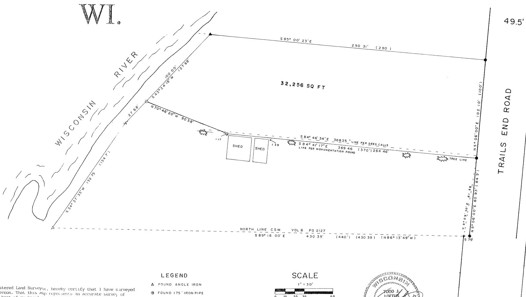
NORTH IS REFERENCED TO THE NORTH LINE OF CSM. VOL 8 PG 2127 BFING AN ASSUMED BEARING OF S 89° 16' 00" E
