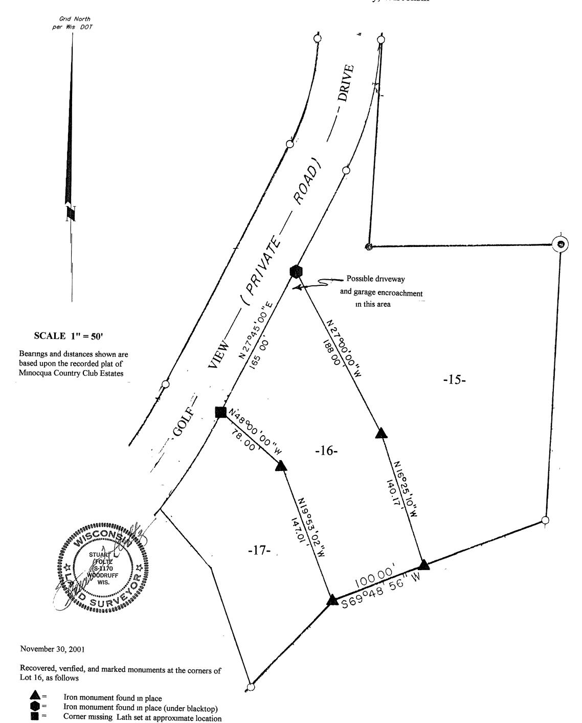
This survey was completed by Foltz and Associates, Inc for the purpose of locating existing lot corners by the order of Mark L Benson, who has executed a written waiver for all other requirements of Wis Adm Code Chap A-E 7 A closed traverse was not made and the minimum accuracy is 1 part in 100 and plus or minus 2°
