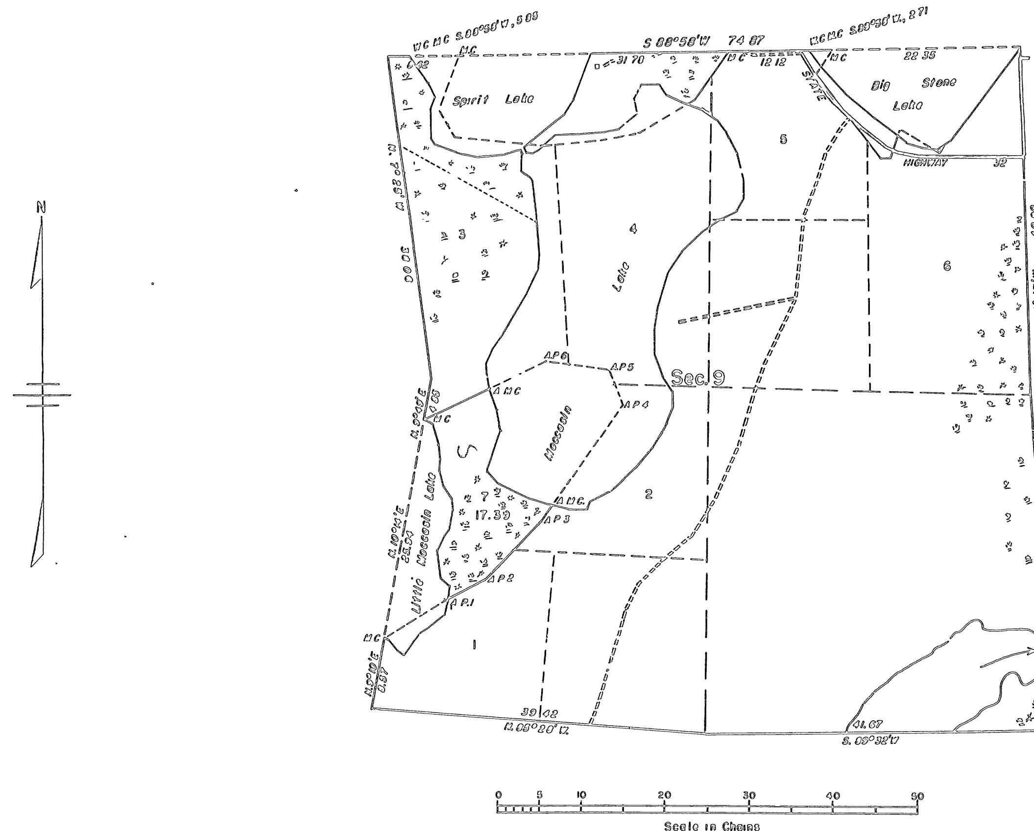
This plan represents a retracement and reestablishment of portions of the original subdivisional lines depicted to restore all corners on the boundaries of Sec. 9 in their original locations according to the best available evidence, and the survey of omitted lands which were erroneously omitted from the original survey and not shown upon the plan approved December 20, 1859.
