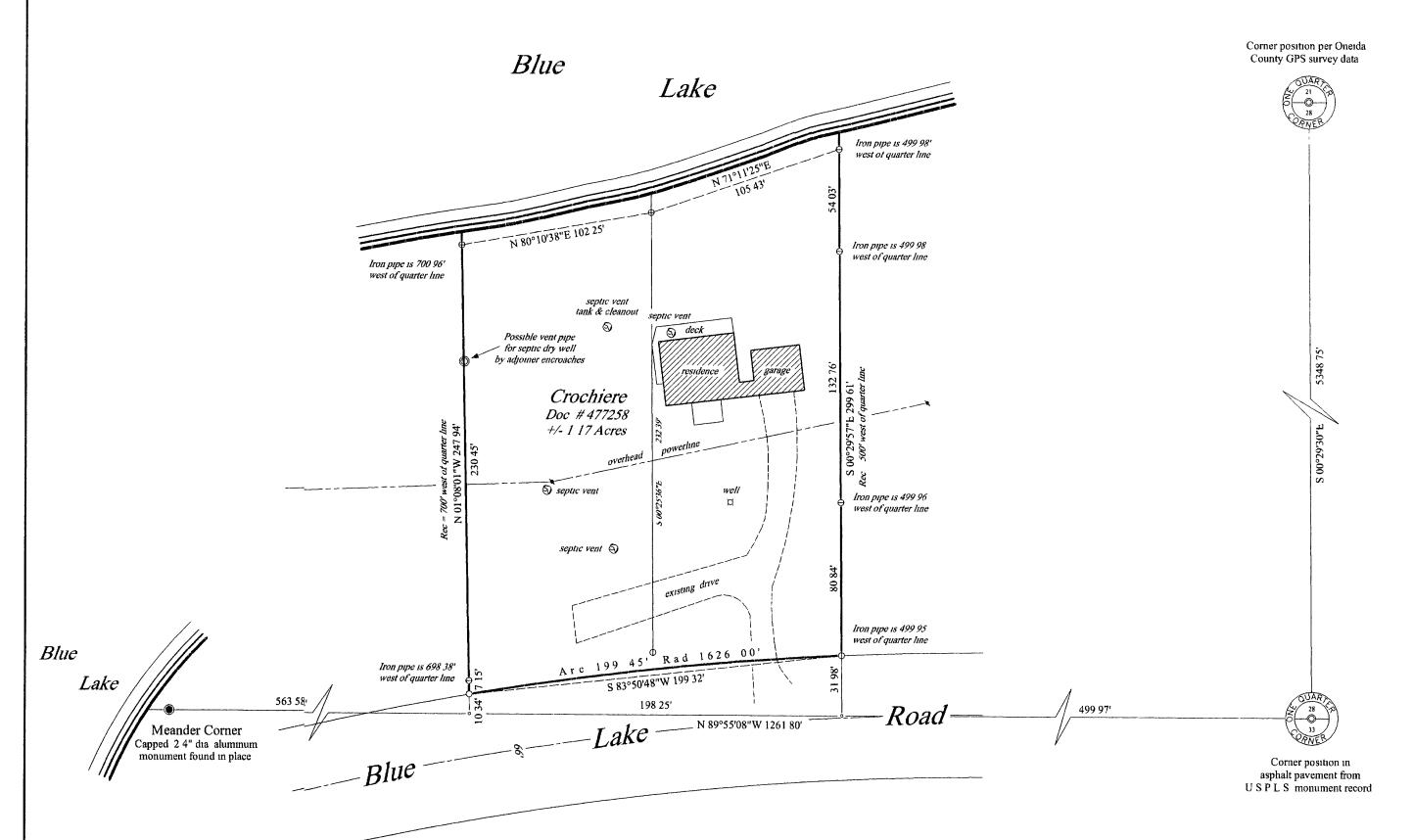
Bearings Oneida County Grid, based on GPS survey data, and referenced to the north-south quarter line, bearing N00°29'30"W
