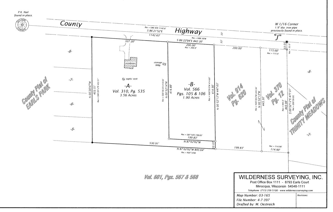
Bearings Oneida County Grid. based on GPS survey data, and referenced to the north line of the NW 1/4 of the NW 1/4, bearing 586°21'52"E
