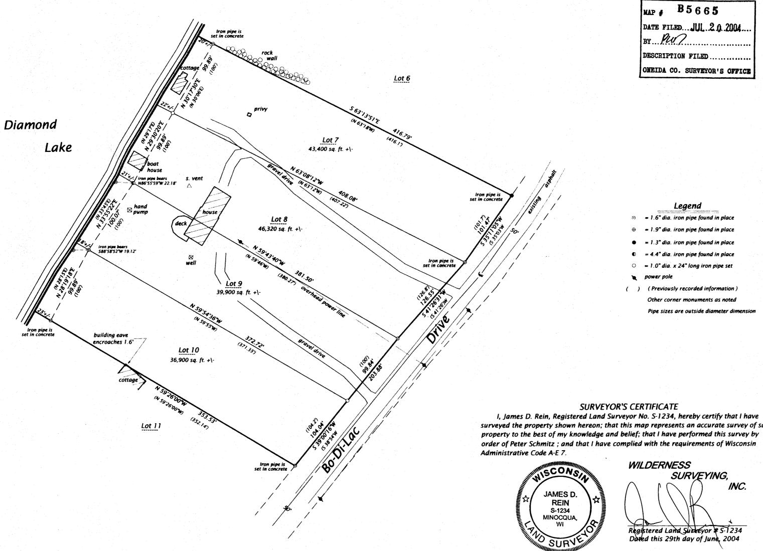
Bearing base recorded, referenced to the south line of Lot 10 bearing N59'26'00'W
