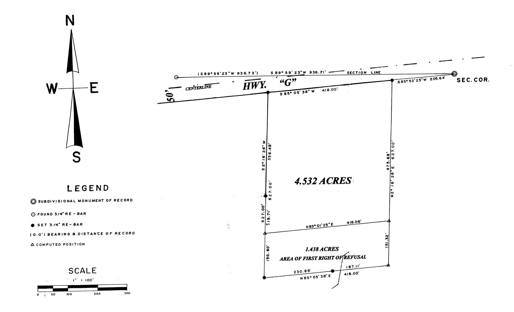
NORTH IS REFERENCED TO THE NORTH LINE OF THE NE' BEING A RECORDED BEARING OF S 89° 59' 23" W.
