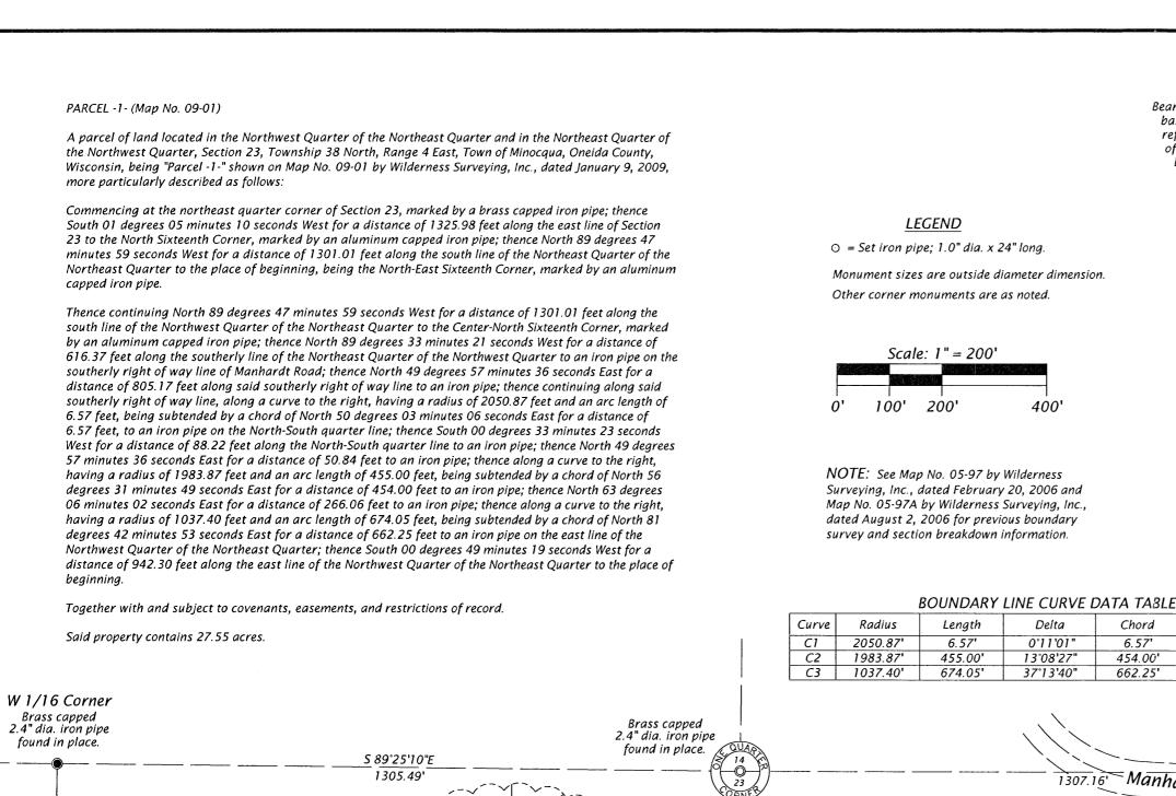
Bearings Oneida County Grid, based on GPS survey data, referenced to the east line of the NE 1/4, Section 23 bearing S 01°05'10"W  $\odot$  = Set iron pipe; 1.0" dia. x 24" long. Monument sizes are outside diameter dimension. Other corner monuments are as noted. NOTE: See Map No. 05-97 by Wilderness Surveying, Inc., dated February 20, 2006 and Map No. 05-97A by Wilderness Surveying, Inc., dated August 2, 2006 for previous boundary survey and section breakdown information.
