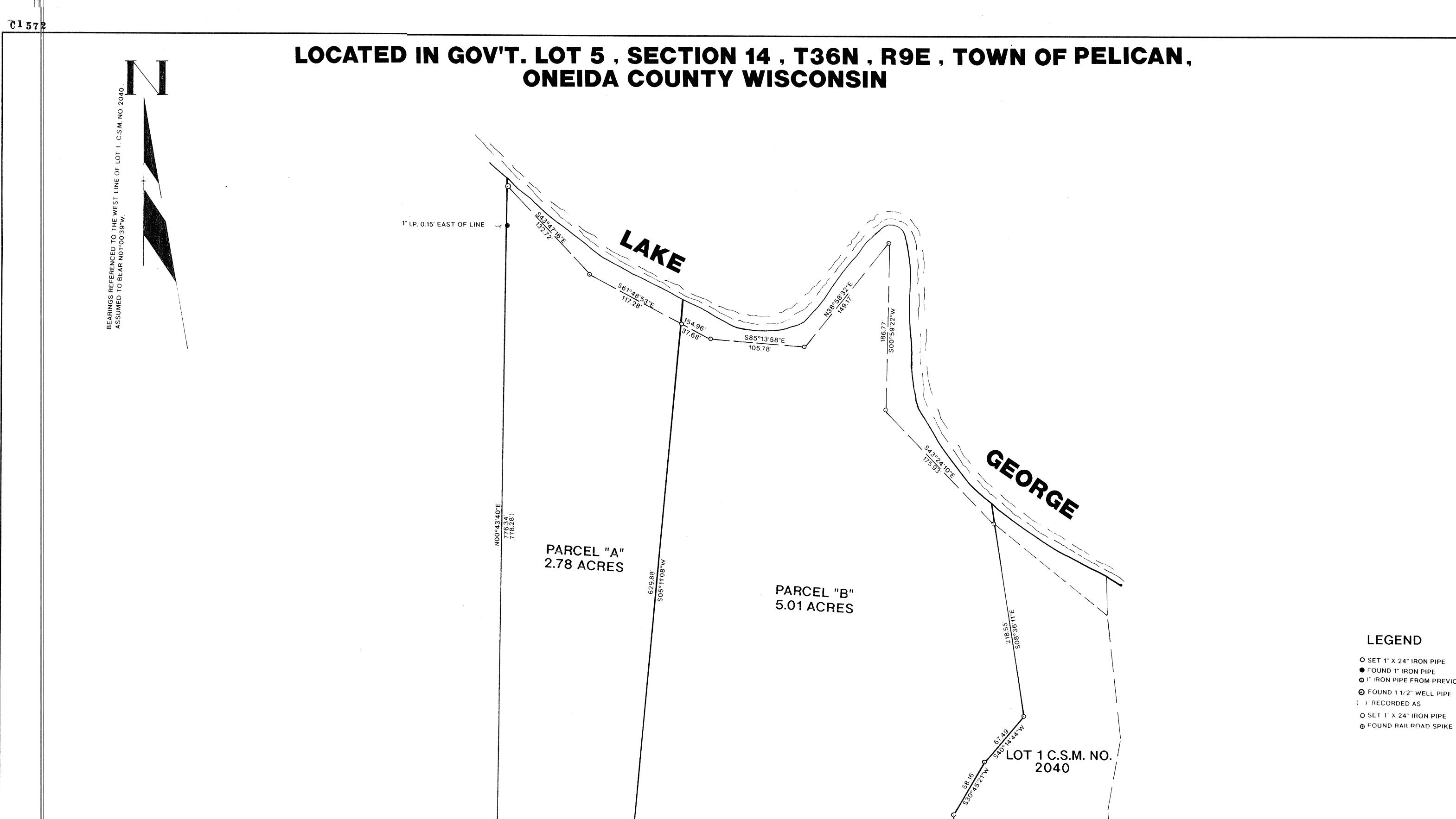
O SET 1" X 24" IRON PIPE ● FOUND 1" IRON PIPE O I" IRON PIPE FROM PREVIOUS SURVEY
