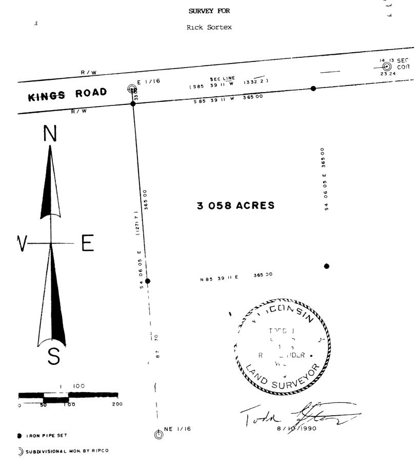
North is reference to the North line of section 23 being a recorded bearing of S  $85^{\circ}$  39  $11^{\circ}$  W
