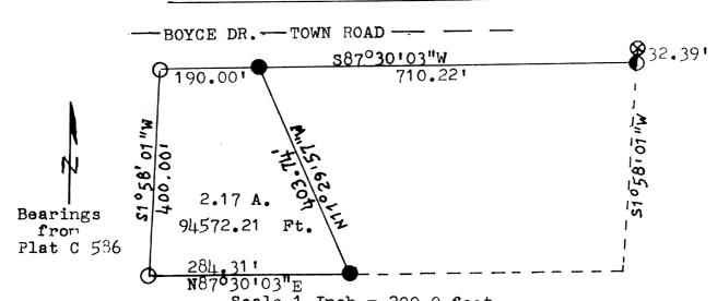
Scale 1 Inch = 200.0 feet ● -Angle Iron O -Channel Iron ● -1 1 1 1 1 Iron Pipe ⊗-N4 Corner
