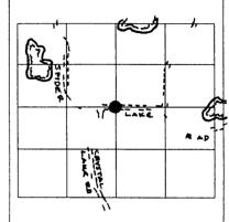
Plan view map of landmark monument location with bearing and distance ties to a minimum of four described witness or reference monuments of concrete natural stone metal live bearing trees or equivalent material or indicate datum & coordinates if tied out using
