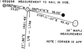
BEARINGS ARE BASED ON THE N -S 1/4 LINE BEARING N 3°-27'-30"E.
