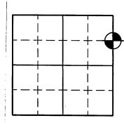
Plan view map of survey landmark location with bearing and distance ties to a minimum of four(4) described witness or THE CIPTURE TO THE CONCRETE, natural stone, metal, live bearing trees or equivalent material and/or described GPS method and precision.
