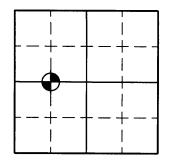
Plan view map of survey landmark location with bearing and distance ties to a minimum of four(4) described witness or reference monuments of concrete, natural stone, metal, live bearing trees or equivalent material and/or described GPS method and precision. 1" = 50'NOTES:
