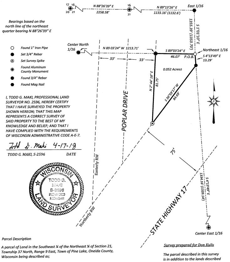
Commencing at the northwest corner of section twenty-one, thence North 88° 26' 39" East for 2258.58 feet along the north section line, thence N 89°13'26" E 1133.16 feet along the north section line, thence S 1°01'10" E 1355.39 feet along the east line of the southeast quarter of the northeast quarter to the Point of Beginning;
