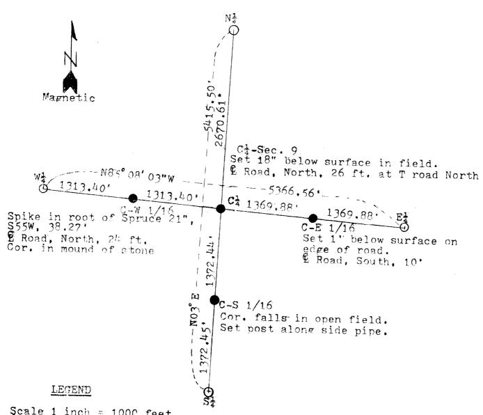
Scale 1 inch = 1000 feet O Corners Found. See certificates for discriptions. Corners Set. 1" Diam. Galvanized Iron Pipe, 3 feet long.
